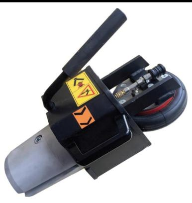
Pneumatically operated, the Core Saver's tapered jaws are simply inserted into the damaged core, no matter how crushed or distorted and the pneumatic action of the jaws returns the core to original its shape allowing the Goldenrod air shaft of chucks to insert easily.
