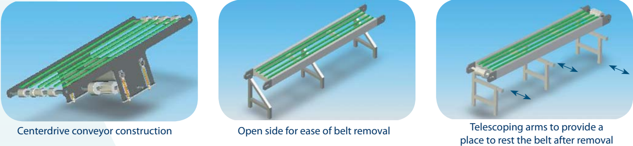
Drawings of Optional Conveyor Designs
