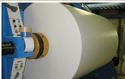
Heavy duty shaftless core chuck
