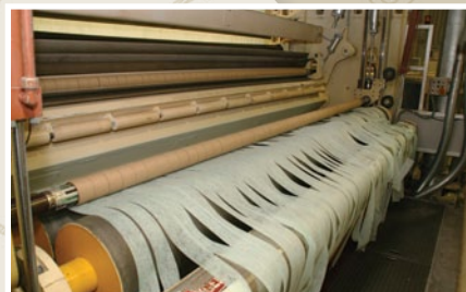
Locked-core shaft in two-drum winder
